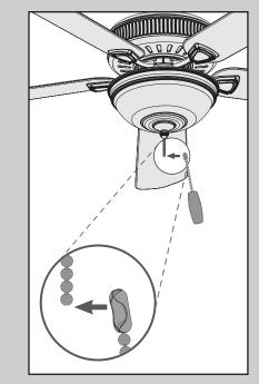
Thread the light pull chain through the hole in the finial and screw the finial onto the threaded rod. Connect the pull chain pendants to the short chains coming from the fan.
